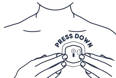
12. Press the button to check the device status. See **INDICATOR LIGHT PATTERN GUIDE** below.
